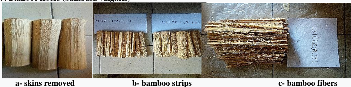
Figure 1: Bamboo defibration steps
