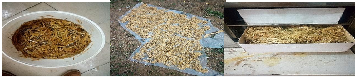
Figure 2: Soaking the fibers in NaOH, drying in the free area for 6 hours and then drying in an oven at 105 ° C for 24 hours.
