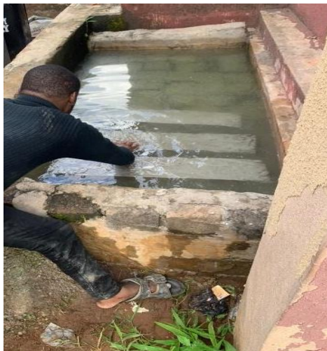
Plate 6: Curing of concrete beam specimens.
