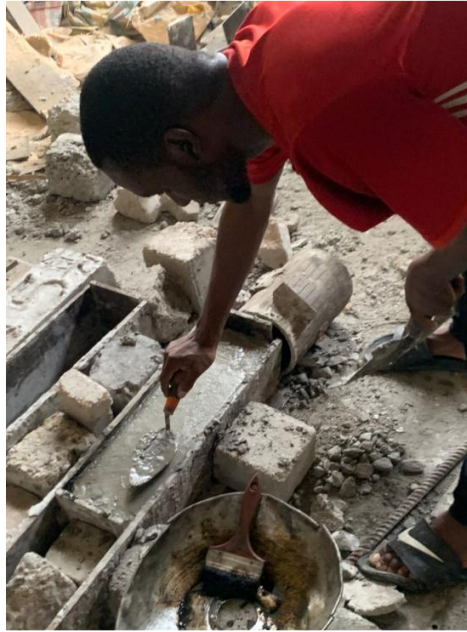
Plate 5: Casting in steel moulds of dimensions 150mm×150mm×500mm.
