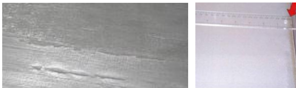
Fig. 7 Strip marking and under-rolled edge
