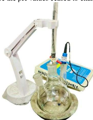
Figure 1. Experimental Setup for pH-metric Titration was used to assess the stability and nature of the resulting metal–ligand complex.
