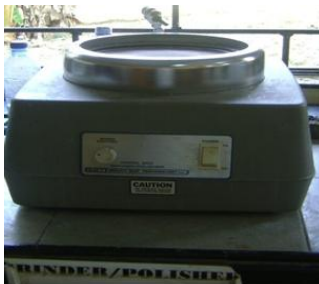
Fig 1: Grinder /Polisher Machine,Model 900,Maker(South bay Technology)
