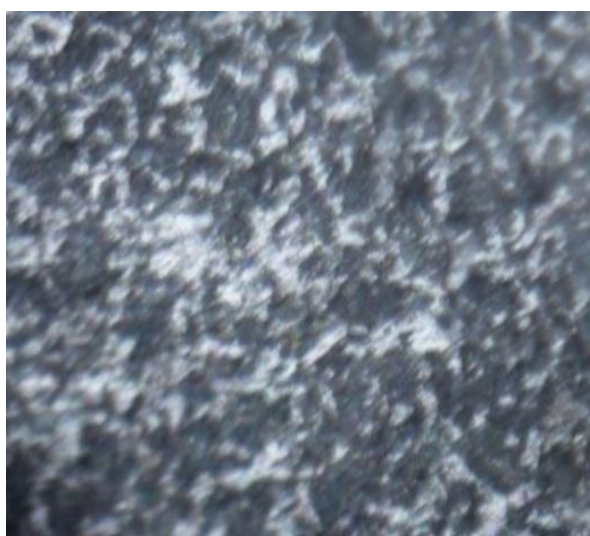
Fig 4 Microstructural View of the tempered Martensite
