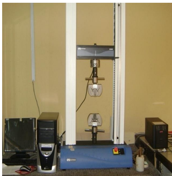
Fig 2: Universal Instron Machine (Model 3369, Maker Instron)
