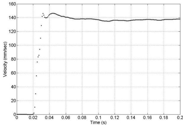
Fig. 3 The piston velocity response of the electrohydraulic servo system without friction load
