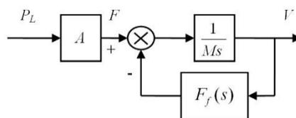
Fig. 5 A block diagram of the friction load
