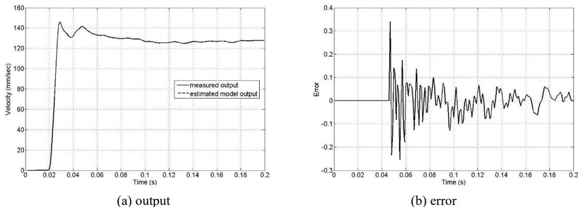
Fig. 7 Comparison measured output and estimated model output (normal force=30kgf)
