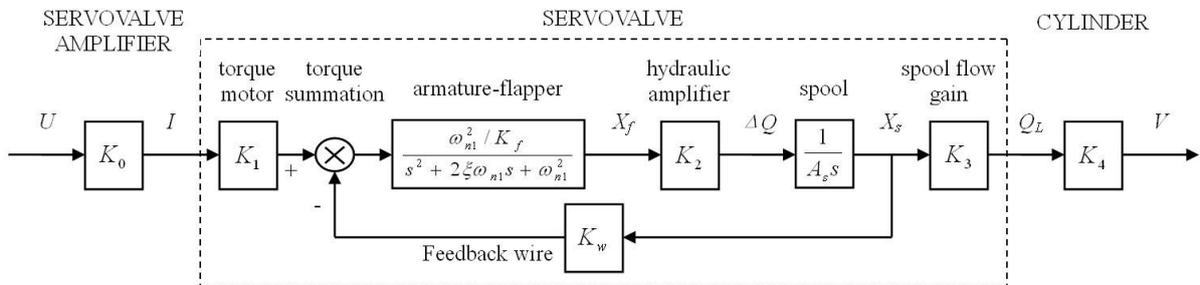
Fig. 2 A block diagram of the electrohydraulic servo system without load
