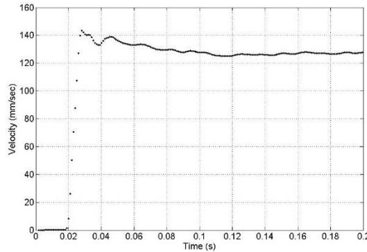
Fig. 6 The piston velocity response with friction load (normal force=30kgf)
