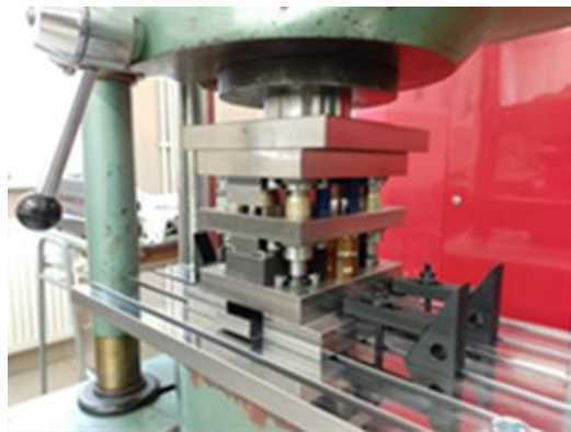
Figure 1 Experimental punch–die set
