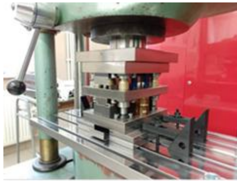
Figure 3 Shearing tool used in the experiment
