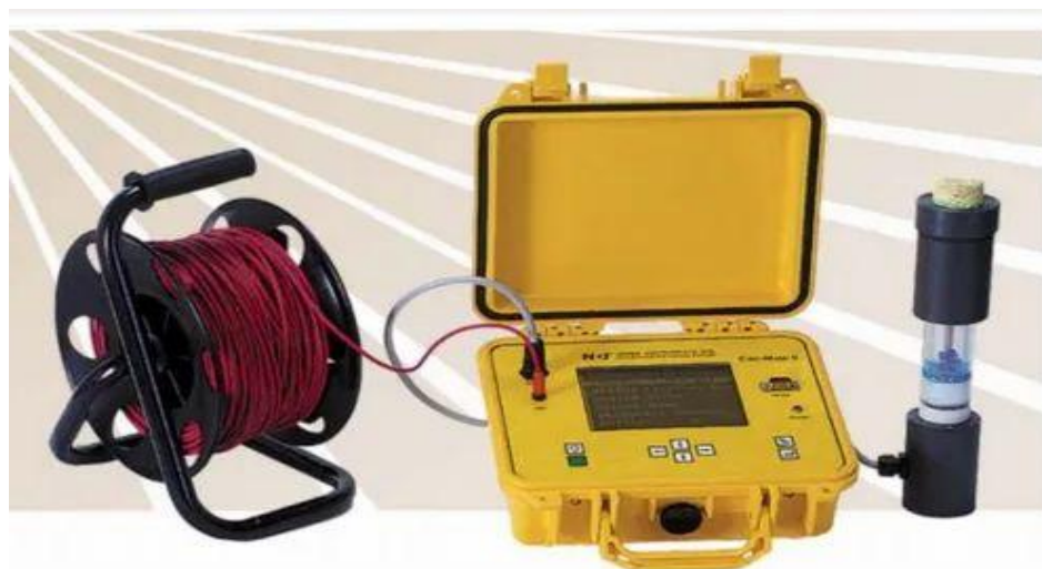
Figure 3: Half Cell Potential Test Equipment for Corrosion Assessment
