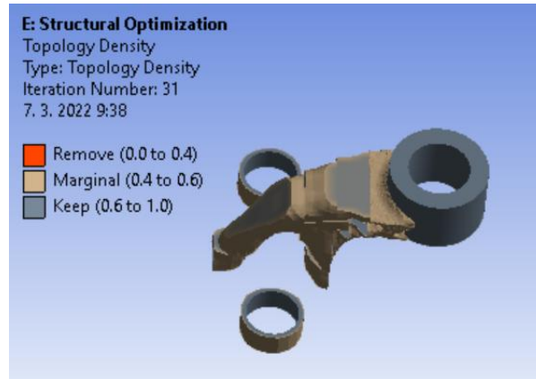
Figure 8 Bracket model created by Ansys topology optimization module
