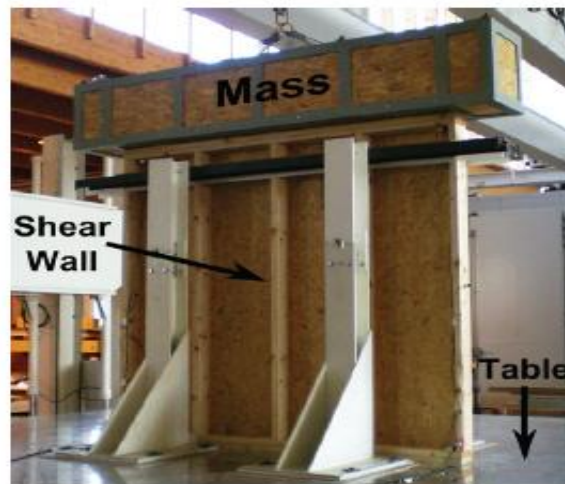
Fig. 2 Dynamic tests set-up on the shake table (FCBA Technological Institute).[6]
