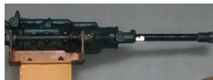
Figure 6.2: Movable plate fitted with jack hammer
