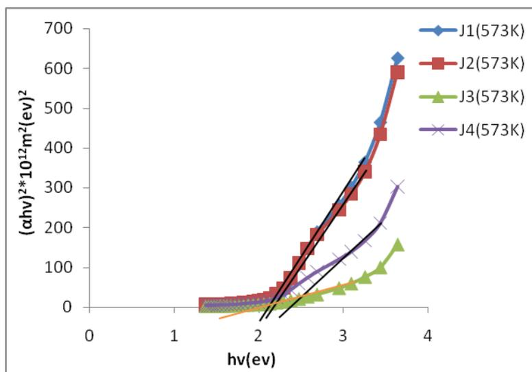
Figure 9b: Plot of  $(\alpha hv)^2$  and  $h\nu$  for annealed CuSe thin films
