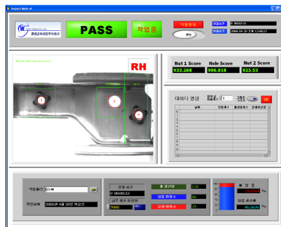
Fig. 12 Main control panel of automatic welding and inspection system using machine vision
