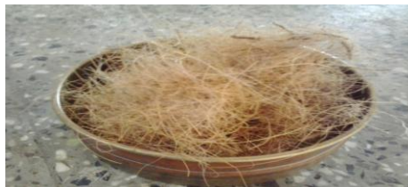
Figure.1. Coir fibers used for reinforcement in clayey soil
