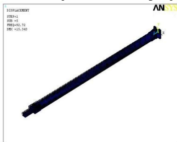
Figure.7.5.1. Modal analysis of Drive Shaft made of Boron/Epoxy
