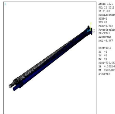
Figure.7.3.3. Natural Frequency of Steel
