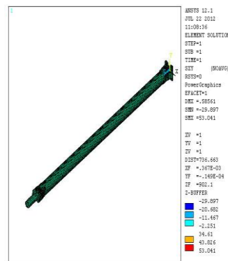
Figure.7.3.2. Shear Stress of Steel
