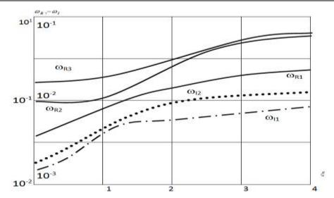
Figure 2.a. Variation of complex Eigen frequencies from the wave number.
