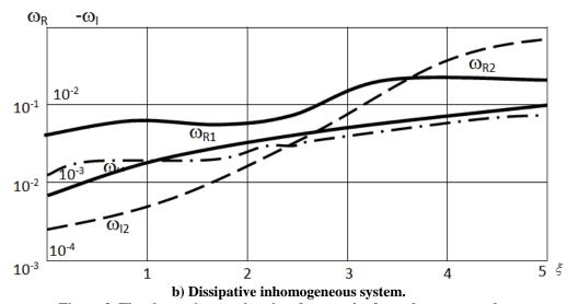
Figure 3. The change in complex eigenfrequencies from the wave number.
