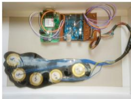
Fig 8. Diagram of diabetic foot ulcer detection & transmission system
