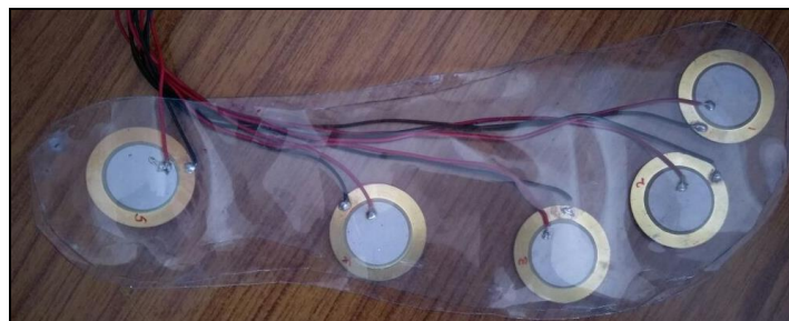
Fig 5. 5 PZT sensors encased in PDMS material
