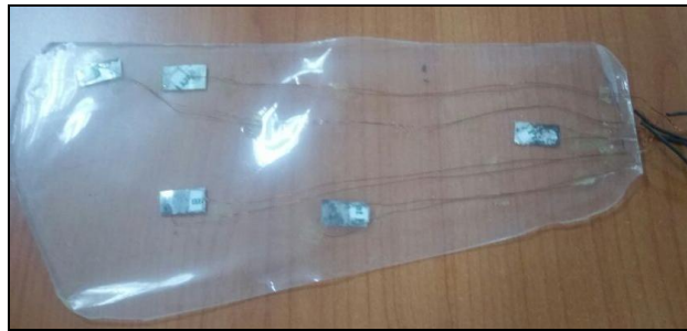
Fig 1. Polyvinylidene fluoride material sensor prototype
