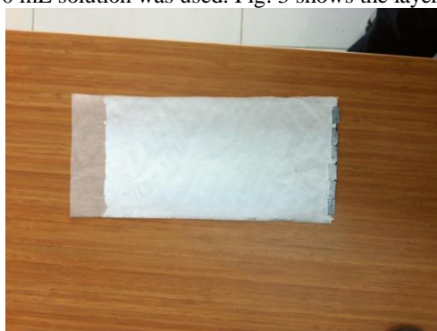
Fig. 3. Nylon 6.6 nanofiber layer
