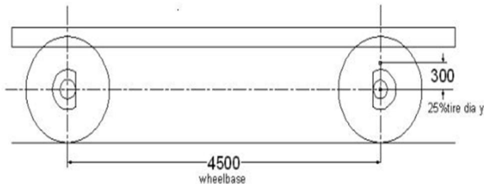
Fig .2 –locating point for upper link axle
