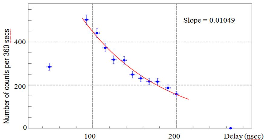
Figure 6: A graph of the number of counts versus the delay in nsec for the coincidence measurement
