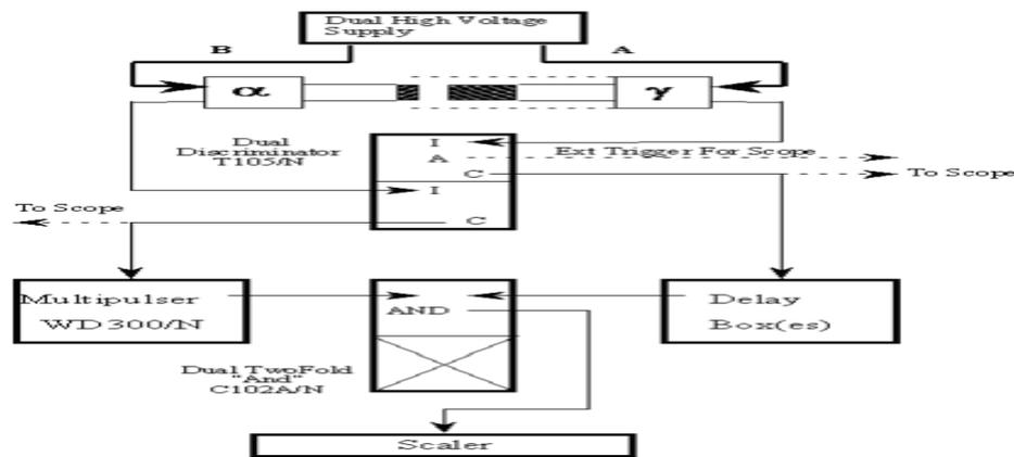
Figure 3: Experimental setup and circuit diagram [3].
