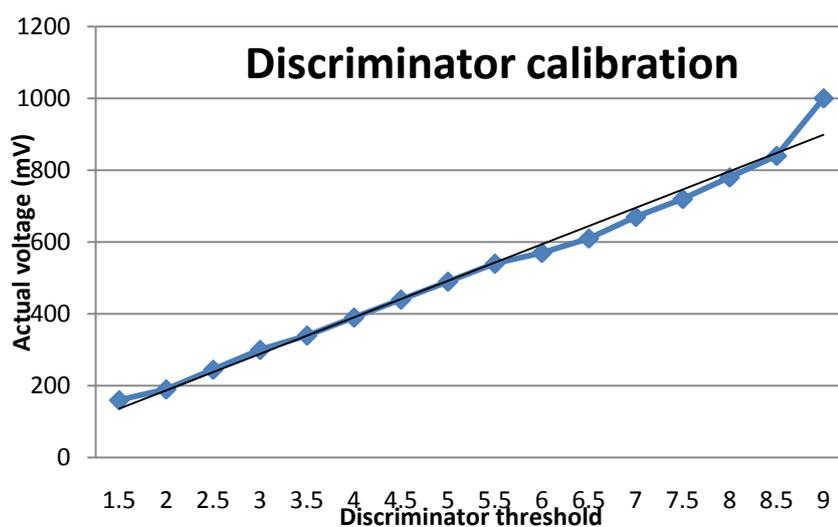
Figure 4: A graph of the actual voltage (mV) versus discriminator threshold for calibrating the dual discriminator.
