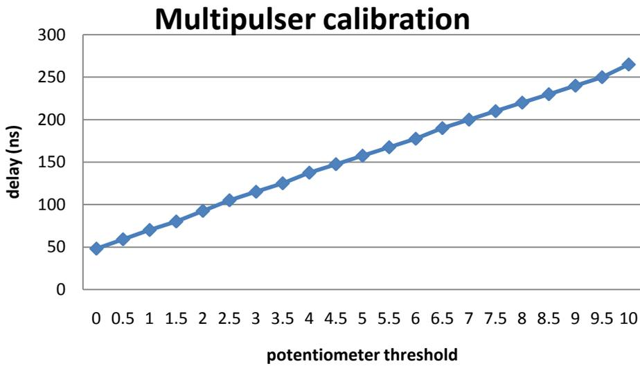
Figure 5: A graph of the readings obtained during the calibration of the multipulser
