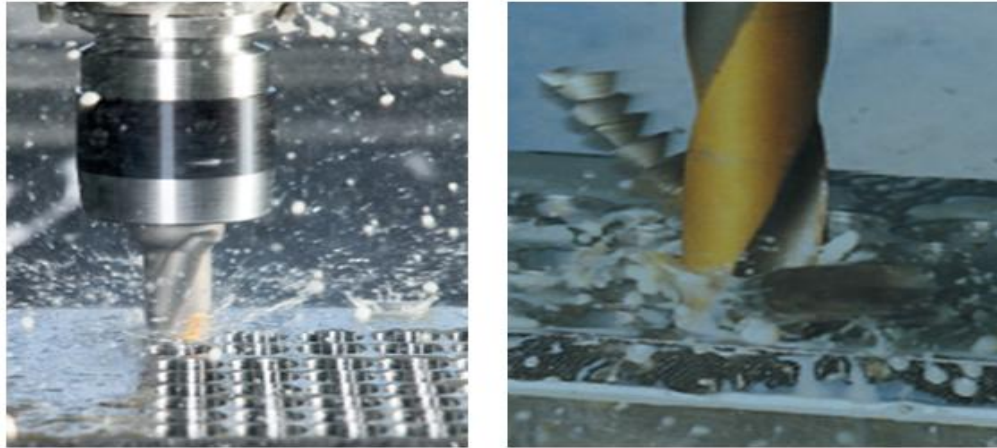
Figure 2: Drilling process during holes in work materials
