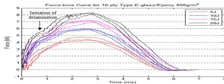
**Figure 7: Force-time curve for 10-ply Type E-glass/Epoxy 800 g/m<sup>2</sup>**
