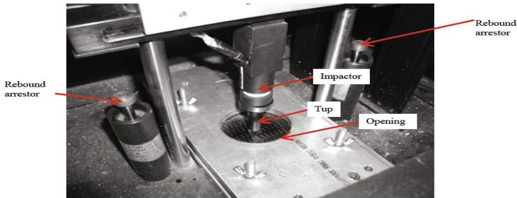
Figure 5: Rebound arrester spring back after first impact
