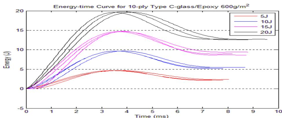
**Figure 8: Energy-time curve for 10-ply Type C-glass/Epoxy 600 g/m<sup>2</sup>**
