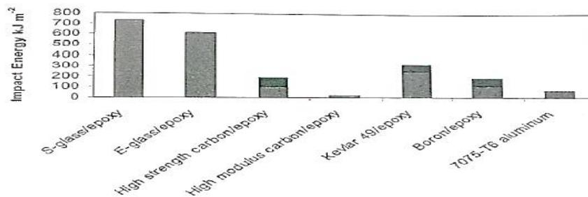
**Figure 1: Charpy impact energy absorption of some materials [9]**
