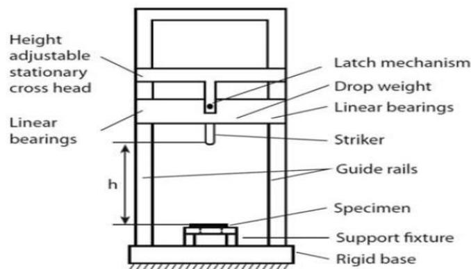
Figure 4: Schematic of drop weight impact test setup [13]
