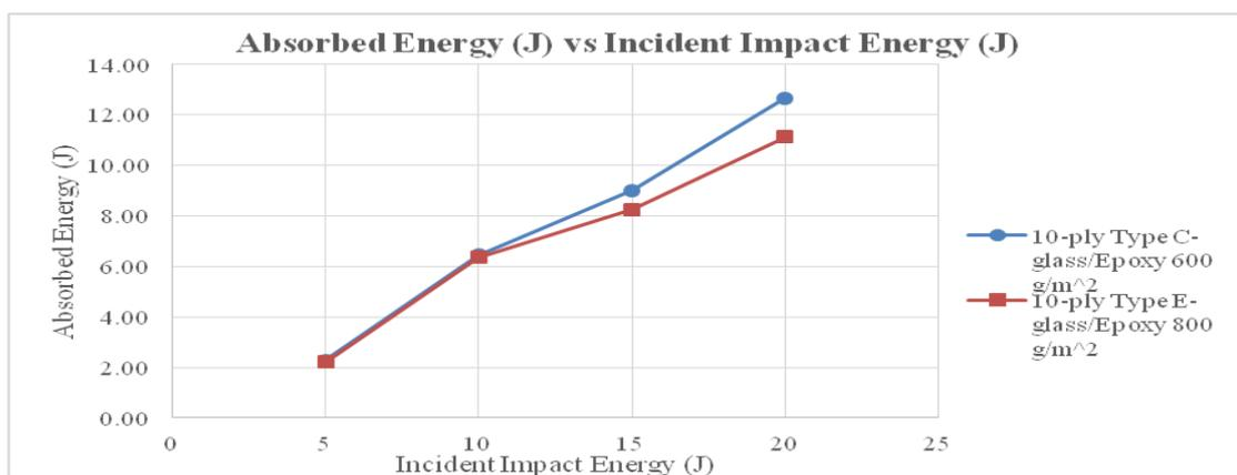
**Figure 13: Variation of absorbed energy and incident impact energy**
