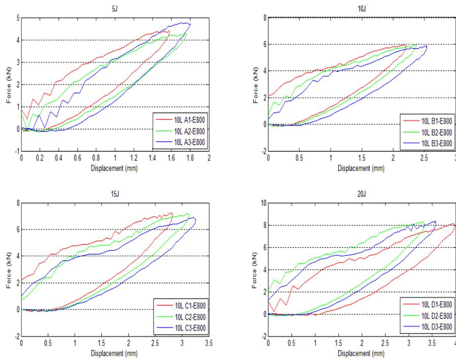
**Figure 11: Force-displacement curve for 10-ply Type E-glass/Epoxy 800 g/m<sup>2</sup>**
