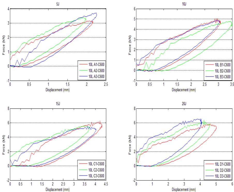
**Figure 10: Force-displacement curve for 10-ply Type C-glass/Epoxy 600 g/m<sup>2</sup>**
