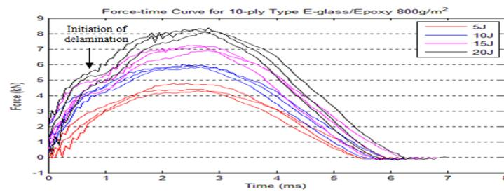
**Figure 7: Force-time curve for 10-ply Type E-glass/Epoxy 800 g/m<sup>2</sup>**
