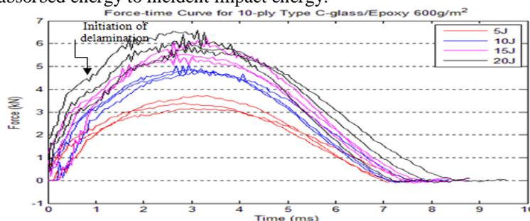
Figure 6: Force-time curve for 10-ply Type C-glass/Epoxy 600 g/m<sup>2</sup>
