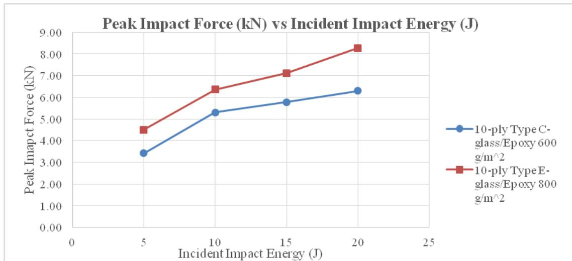
**Figure 12: Variation of peak impact force and incident impact energy**
