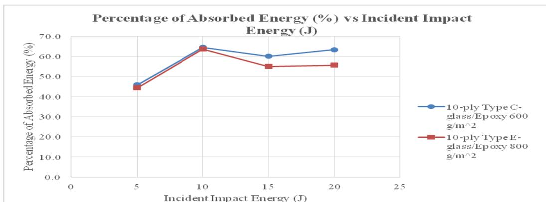
**Figure 14: Variation of percentage of absorbed energy and incident impact energy**
