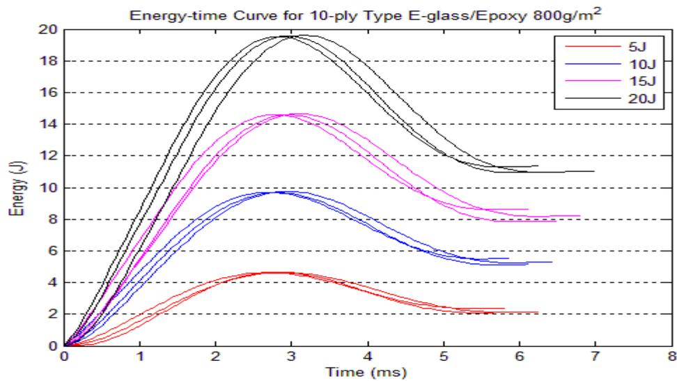
**Figure 9: Energy-time curve for 10-ply Type E-glass/Epoxy 800 g/m<sup>2</sup>**
