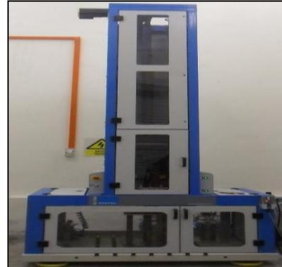
Figure 3: Imatek IM10 ITS drop weight impact tester
