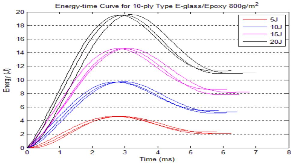
**Figure 9: Energy-time curve for 10-ply Type E-glass/Epoxy 800 g/m<sup>2</sup>**
