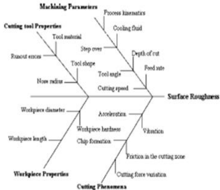
Figure 2 : Fishbone Diagram showing parameters affecting surface roughness
