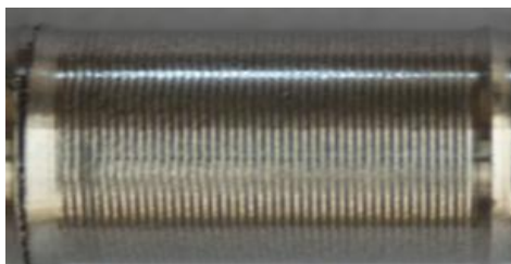
Fig.7a: Rough Surface Roughness on SS 316L Pipe before optimization
