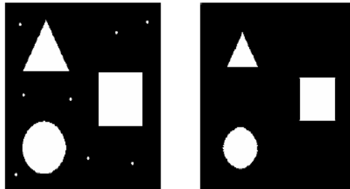
Figure 2.6: Binary Erosion Example
