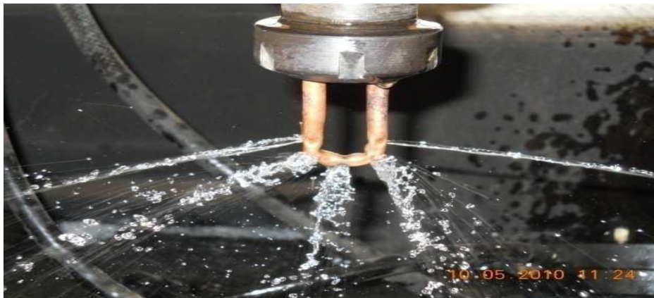
Figure 10 : Introduction of Dielectric Fluid in EDM process
