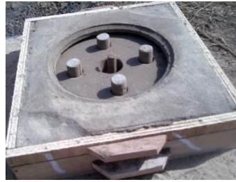
Fig. 12: Picture of the cheek and drag subassembly showing dried cores in the core print cavities prior to casting
