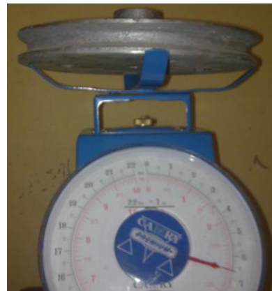
Fig. 16: Cast pulley being weighed on a scale after fettling
