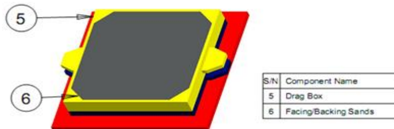
Fig. 6: Place the drag box on the cheek; pour and ram facing and backing sands consecutively
