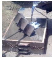
Fig. 14: Pouring of molten aluminium into the sand mould
