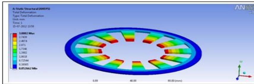
Figure 2: Deflection for slotted Belleville spring
