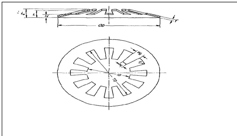
Figure 1: A Slotted Belleville Spring
