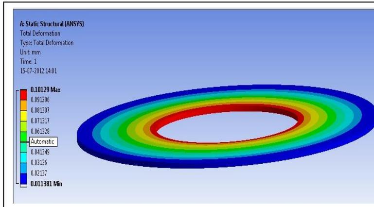
Figure 4: Deflection for Belleville spring of same dimensions without slots
