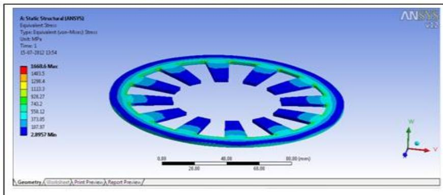
Figure 3: Von-misses Stress for slotted Belleville spring
