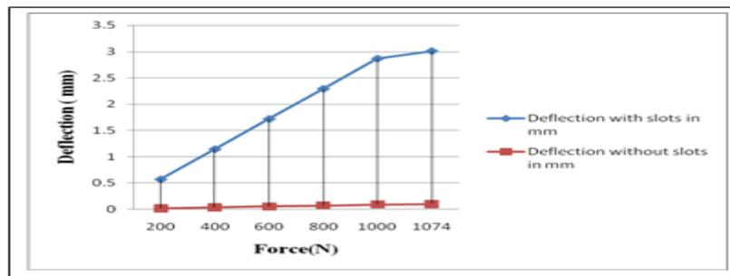
Figure 7: Load – Stress Characteristic for Belleville spring with and without slots
