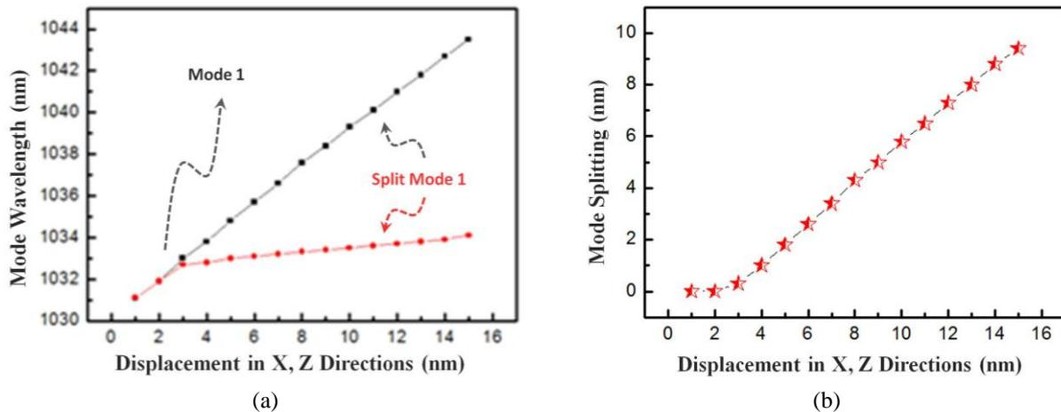
Figure 5. a) Variations of wavelength along the fundamental confined mode which undergoes splitting, and b) splitting values for different air-hole displacements.
