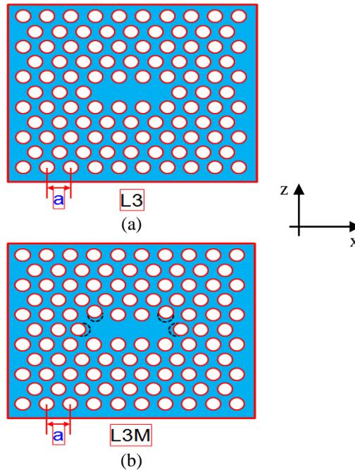
Figure 2. Schematic of top view of a) the normal L3 PhC-DNCs, and b) displaced air-holes and a typical direction of their displacements; L3M is the L3 with modifications.
