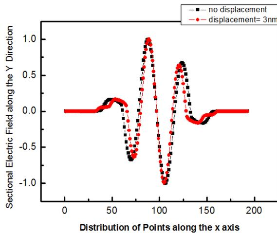
Figure 4. Electric field distribution profile of the modes which shown in the previous figure, across the L3 nanocavity, along the x axis ( $z=0$ ) for normal L3 and modified L3M with 3 nm air-holes displacements shown in the Fig.2.
