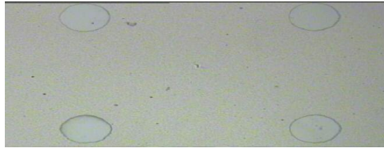
Figure 7: Shows patterning of Al before etching process. Etching anymore and as it shows in fig. 9, there will be under-etching in process due to increasing temperature above 250 °C.
