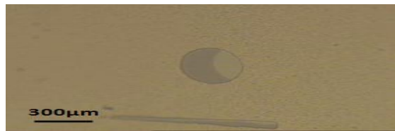
Figure 8(a): Shows vertical etching of SiC used SF 6 and O 2 gases.
