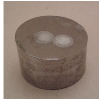
Fig5. Marks of Argon Gas on Specimen EN-24
