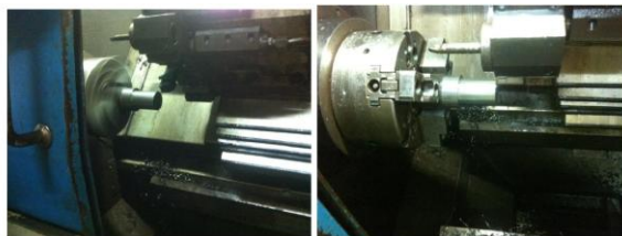
Fig9. Pictorial view of machining of workpiece EN-24 on CNC Machine
