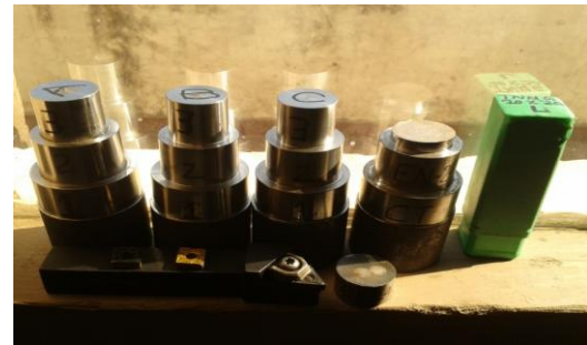
Fig11. Overview of three finished specimens of EN-24 as per dimensions desired using three different tool inserts on CNC machine.
