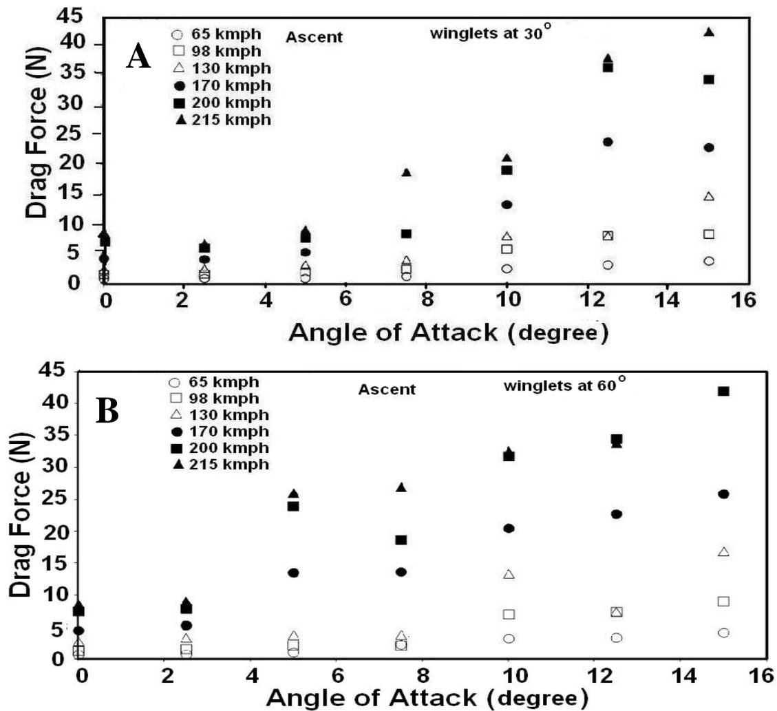
Figure 7. The drag versus angle of attack of a airplane with winglets during ascent. Winglet angle (A) 30° and (B) 60°.
