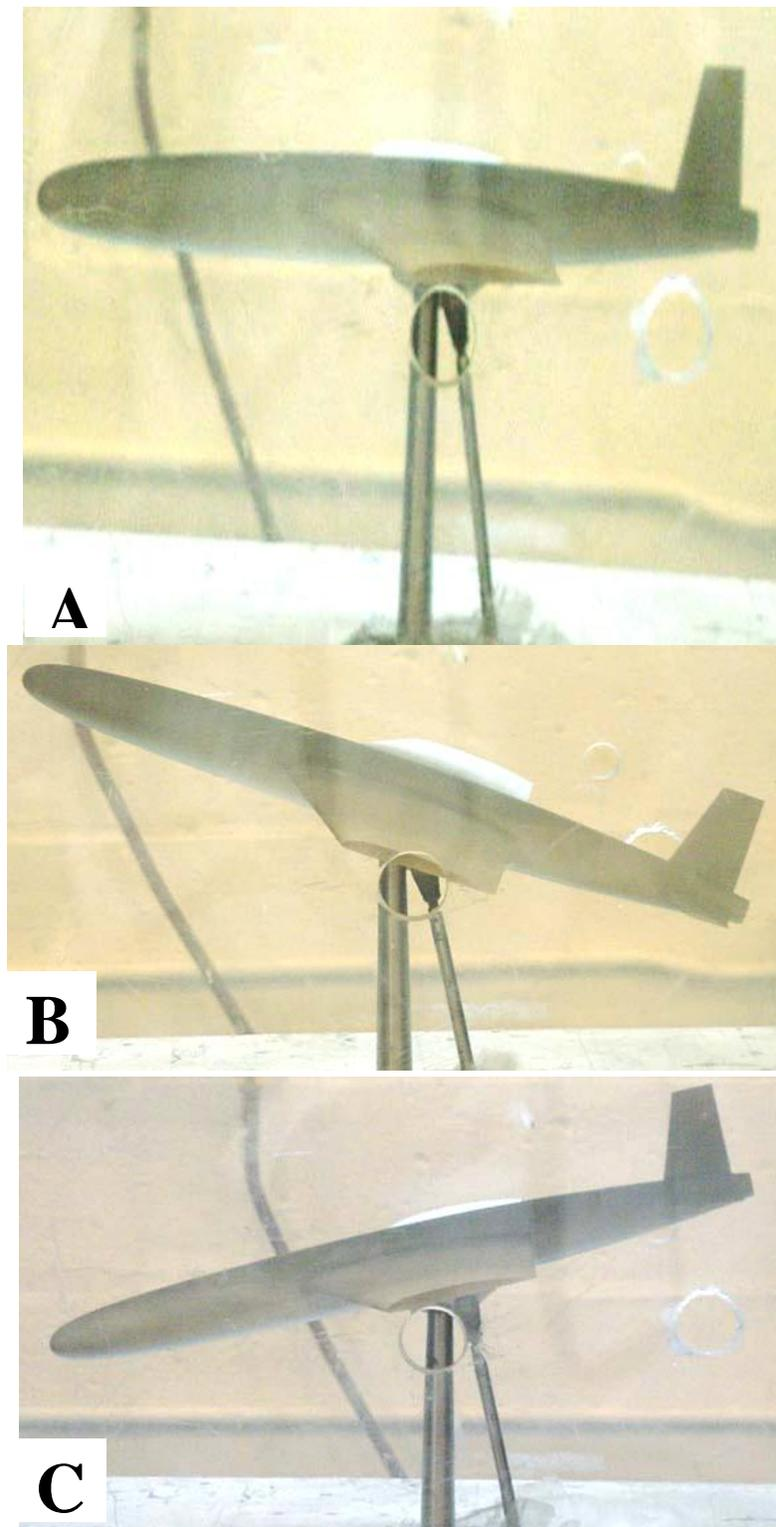
**Figure 4.** Model airplane with solid wings during wind tunnel experiments. Angle of attack (A)  $0^\circ$ , (B)  $15^\circ$  ascending and (C)  $15^\circ$  descending.
