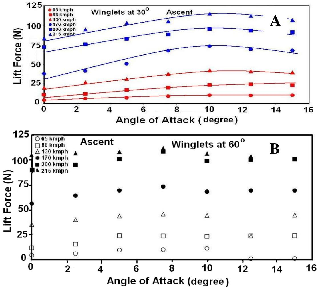
Figure 6. The lift force versus angle of attack of an airplane with winglets during ascent. Winglet angle (A) 30° and (B) 60°.
