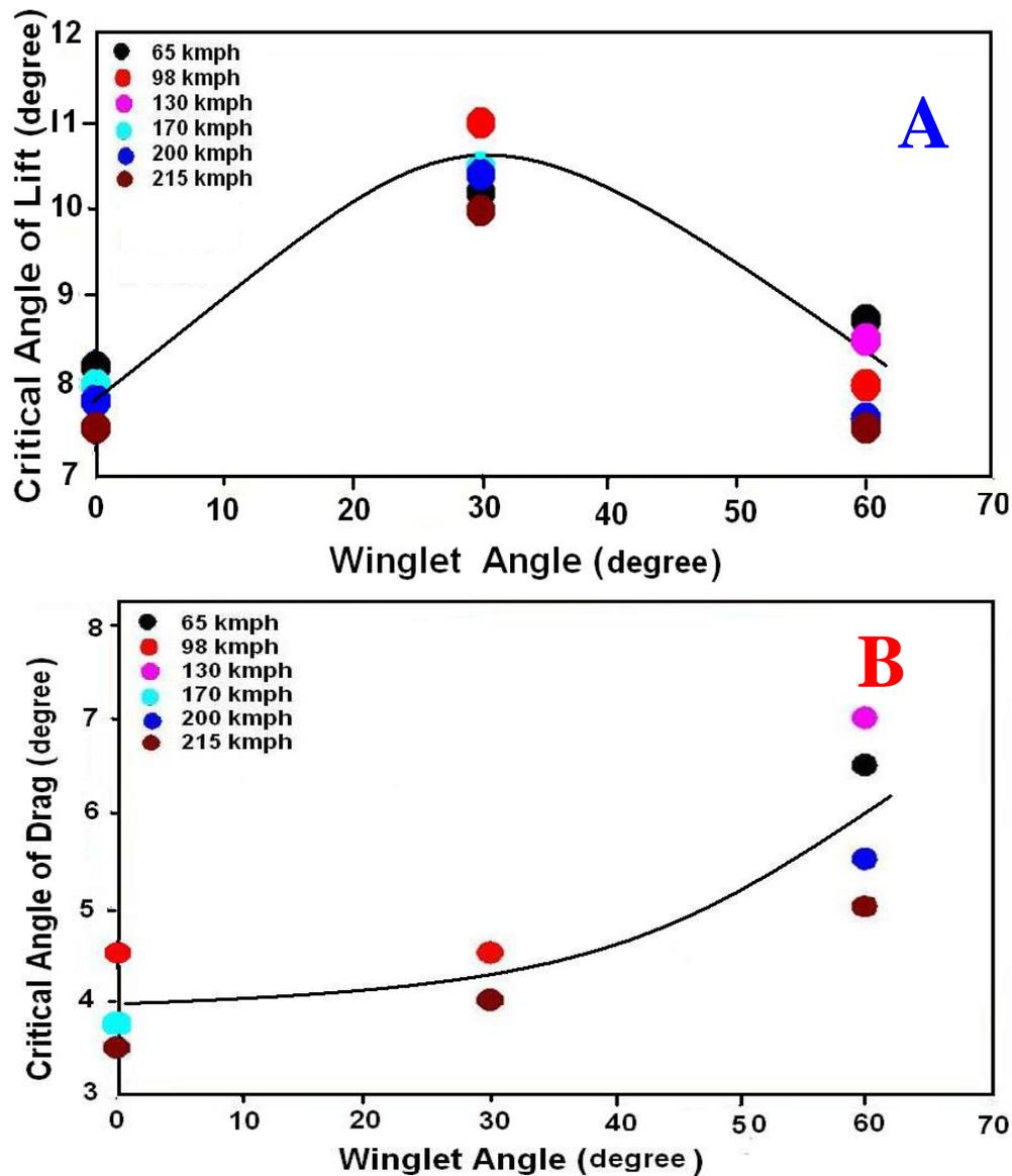
Figure 8. The critical angle of attack of (A) lift and (B) Drag versus the winglet angle of an airplane during its ascent.
