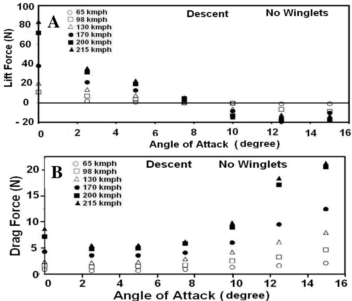
Figure 5. The (A) lift force or (B) drag force versus angle of attack of an airplane without winglets during descent.
