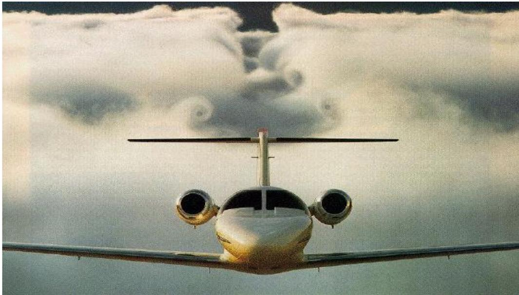
Figure 2. Typical airplane in flight with the vortex formed behind the airplane. (ref. 3)
