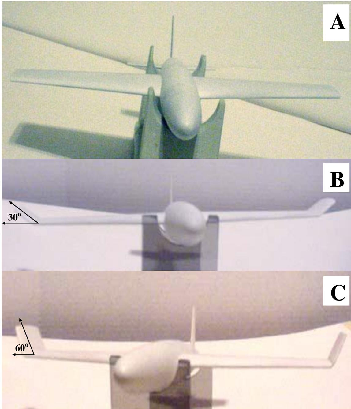
**Figure 3.** Typical airplane models (A) no winglets and (B, C) solid winglets attached at  $30^\circ$  and  $60^\circ$  to the plane normal to the fuselage respectively.
