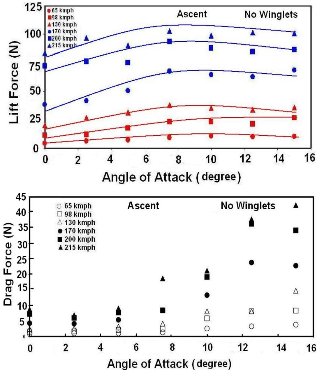
**Figure 4.** The (A) lift force or (B) drag force versus angle of attack of an airplane without winglets during ascent.
