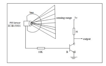
The proposed system basically controls illumination intensity of a lighting device according to user movement and brightness of surroundings [4]. That is, when the maximum value of illumination intensity of a lighting device is Lmax and the minimum value is Lmin, the illumination intensity becomes Lmax, if user movement is detected and becomes Lmin, if user movement is not detected for certain period time[8][9].
