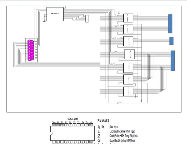
**B.74LS154 4-LINE TO 16-LINE DECODER/DEMULTIPLEXER:** Each of these 4-line-to-16-line decoders is used to decode four binary-coded inputs into one of sixteen mutually exclusive outputs when both the strobe inputs G1 and G2 are LOW. The demultiplexing function is done by 4 input lines to address the output line, by sending data from one of the strobe inputs with the other input LOW. These demultiplexers are ideally suited for implementing high-performance memory decoders.
